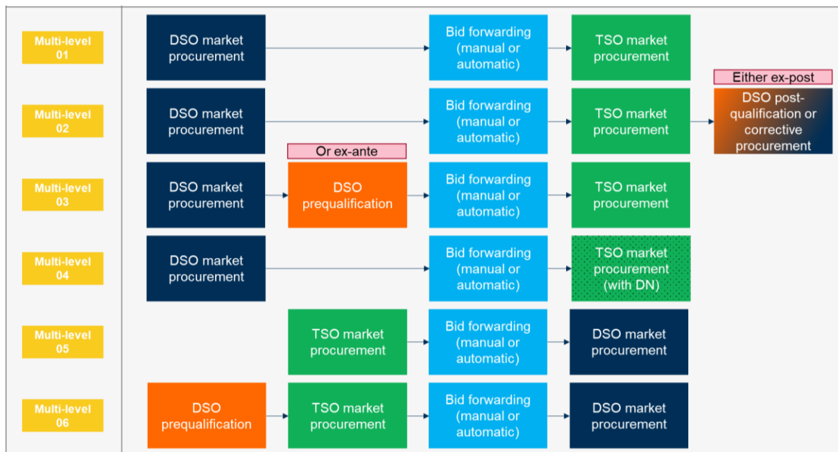
Figure 3-5: TSO-DSO coordination model when both TSO and DSO procure flexibility in separate markets (multi-level market models).
