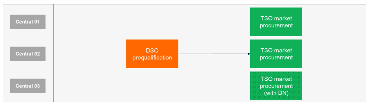
Figure 3-4: TSO-DSO coordination model when the TSO is the only one procuring flexibility (central market models).
